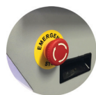
EMERGENCY STOP BUTTON
